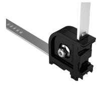
The robust latching points with 8 mm pins in stainless steel are good for forces up to 1300 kgs (2800 pounds) per piece. The latching point is bolted on the frame and welded on the door. Their special shape makes it easy to open and close the door. Cut-outs in the door are used to align the latching points during welding.
