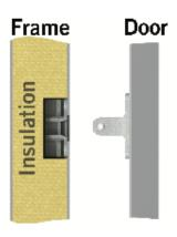
The locking points consists of a protruding frame part and a receptacle hidden on the inside of the door.
